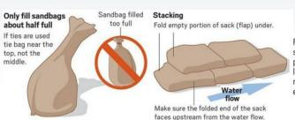
Freestanding sandbags should be stacked in a pyramid. Stagger them like bricks so they are not directly on top of each other.
